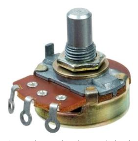
A **potentiometer** is a three-terminal resistor with a sliding or rotating contact that forms an adjustable voltage divider. If only two terminals are used, one end and the wiper, it acts as a variable resistor or rheostat.
